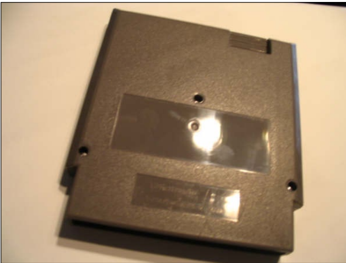
Top Left: As you can see, there is no adhesive residue where a back label would normally be. Top Right: Finding EPROMs when opening the case is a very good thing, if it says Nintendo.
