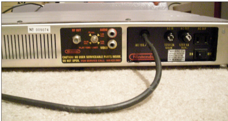
Left: The back of the M8, housing outputs in both RF and AV format.
