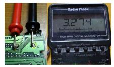
the 2 points on the back of the PCB, where the bands come thru. If all is well, you should get a reading of ~3.3V.
