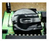
**Step 3**: Wrap each end of the tape up over the top clip, pulling somewhat snuggly to ensure a tight connection.
