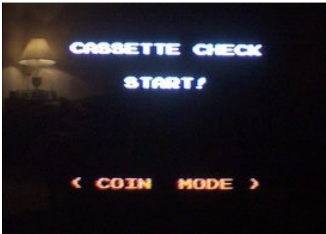
Above: When it first powers on, it tests the carts. This is the first screen. Right: Here is what a cart looks like. It's a regular NES cart case, but black.
